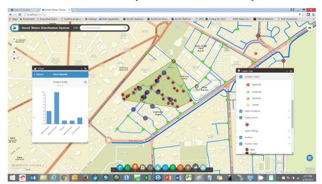
Smart Water Distribution System – Dashboard for monitoring NRW
